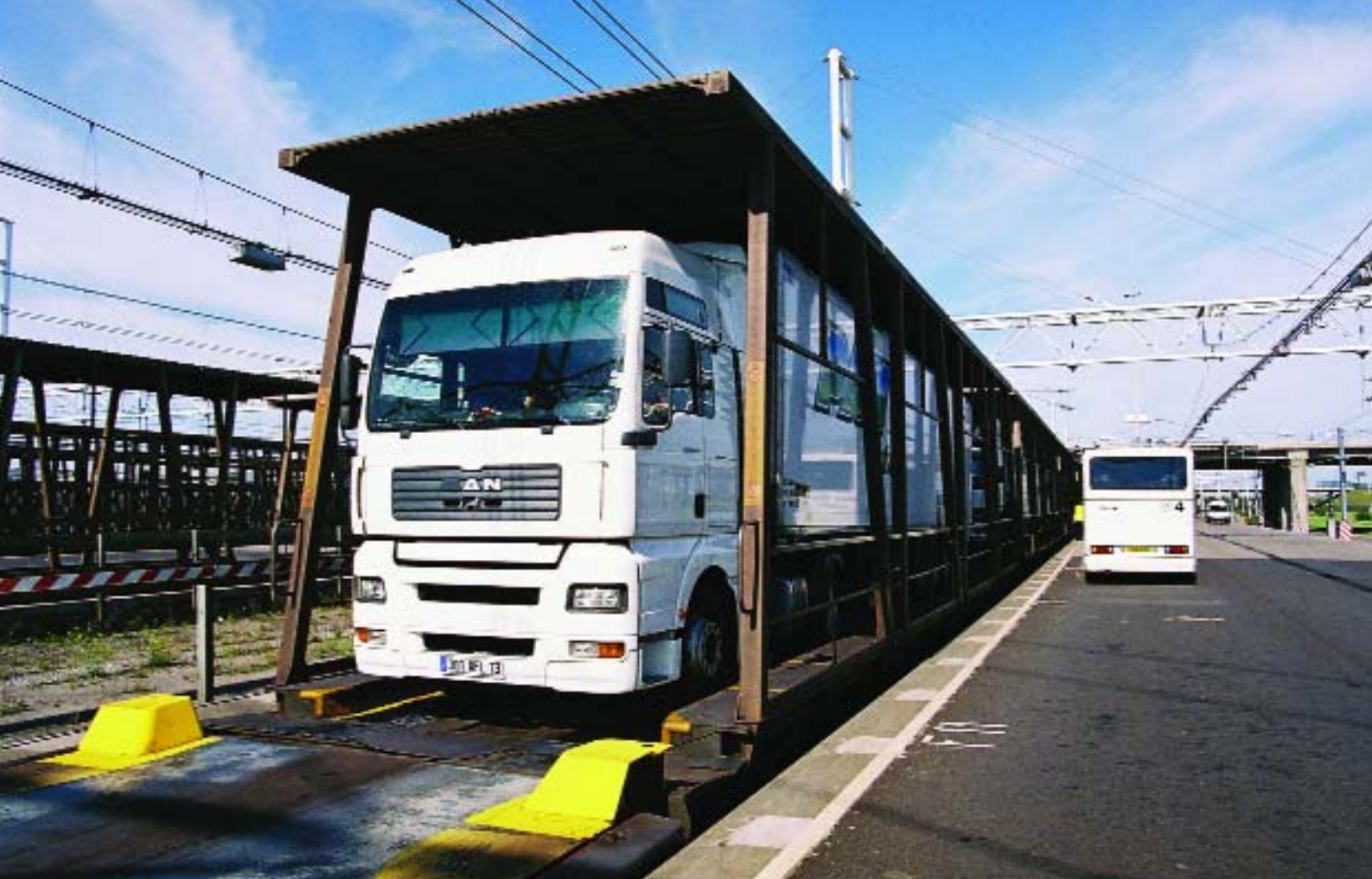
Rolling roads already operate through the Channel Tunnel (above) and in parts of Switzerland. The proposed Woodhead Line would keep lorries off roads in the Peak District.
