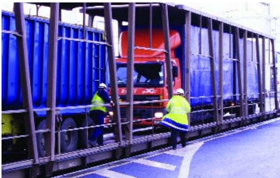
Trucks load onto an Arbel-type Eurotunnel truck shuttle to be transported underneath the Channel.
