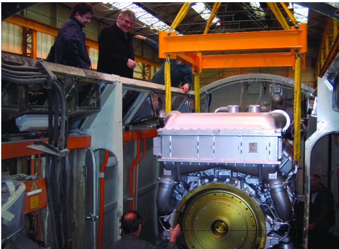
An MTU 16-cylinder, 1,800rpm engine is dropped into a First Great Western HST power car as part of Angel Trains' £1.4m HST life-extension trial. First Group's chief executive, Moir Lockhead (top, centre) looks on.
